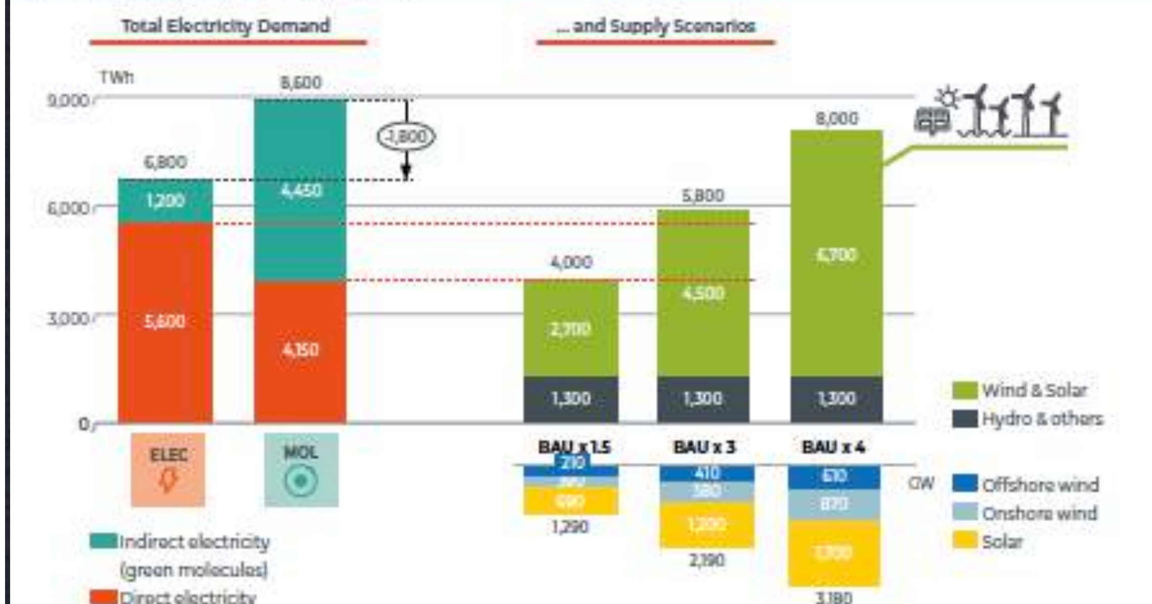
FIGURE 2: STRONG ELECTRIFICATION OF END USE (AS UNDER THE ELEC-PATHWAY) SAVES UP TO 1,800 TWh AT THE EUROPEAN LEVEL COMPARED TO THE MOL-PATHWAY. DIRECT ELECTRICITY DEMAND UNDER THE ELEC-PATHWAY INCREASES BY 70% COMPARED TO TODAY'S DEMAND. A TRIPLING OF TODAY'S RES EXPANSION RATE IS NEEDED TO MEET THIS DIRECT ELECTRICITY DEMAND
